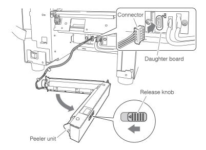
(10) After positioning the peeler unit on the printer using the alignment pins on the peeler as a guide, fix the unit to the printer using the screw supplied. Then close the peeler.
