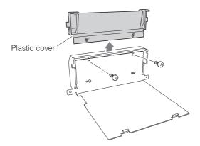
(7) Attach the peel guide plate to the front center cover taking care not to over-tighten the screws as they are threaded in plastic. (2 screws)
