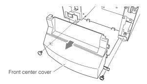
(6) Remove the plastic cover from the front center cover that you have removed. (2 screws)
