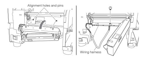
(11) Align the two tabs on the bottom of the 'front center cover' to the slits of the printer as it is slid in to the printer. The bottom plate of the front cover needs to be held up from below to ensure a good fit. Attach the front center cover from step 5 in its original position. (3 screws, of which 1 is an accessory to the unit)
