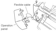
(4) Remove the front right cover on the front of the printer. (2 screws)
